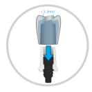
The diameter of the screw channel for the VICARBO® screw must be greater than 3.3mm for the RN platform.
