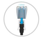
The diameter of the screw channel for the VICARBO® screw must be greater than 3.0mm for the SN platform.
