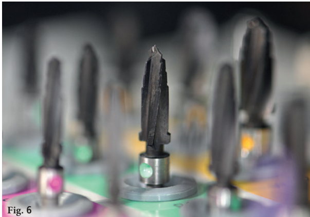
Figure 6: XT profile drills color-coded with carbon coating. Figure 7: Pilot and profile drills: intrabony length of 10 mm plus 0.6 mm in the neck area.
